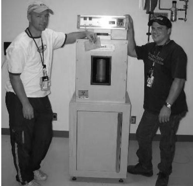
Figure 2: Typical self-shielded Cs-137 blood irradiator.
