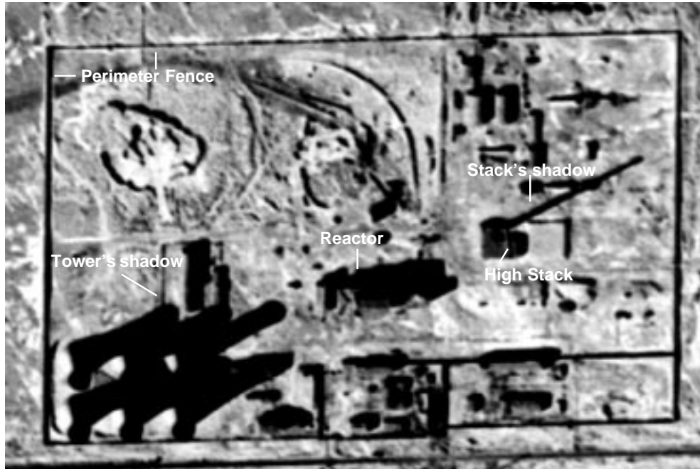
Figure 4b: Declassified US CORONA satellite imagery of Jiuquan plutonium production reactor. (CORONA mission 1108-1, December 9, 1969). From this photo, the perimeter fence and high stack are made visible through their shadows.
