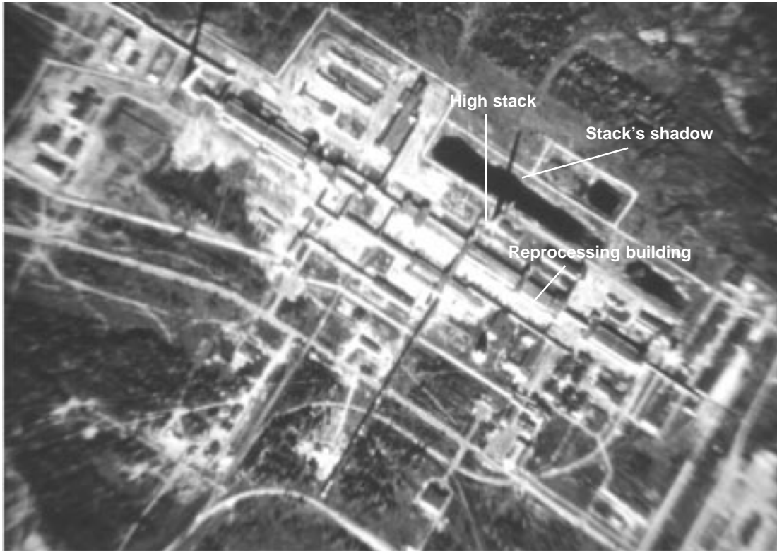
Figure 1: Declassified US CORONA satellite image of the reprocessing plant at Tomsk-7, Russia. (CORONA mission 1115-1 on September 15, 1971, KH-4B system, six-foot spatial resolution). The long reprocessing building and the high stack (through its shadow) are clearly visible. Source: US Geological Survey, EROS Data Center, Sioux Falls, SD.
