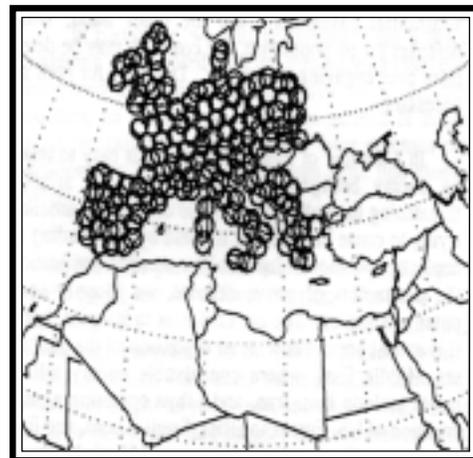
**Figure 1. Coverage of Europe against a North African Missile Threat (from Libya) Using 100 Autonomous Batteries**
